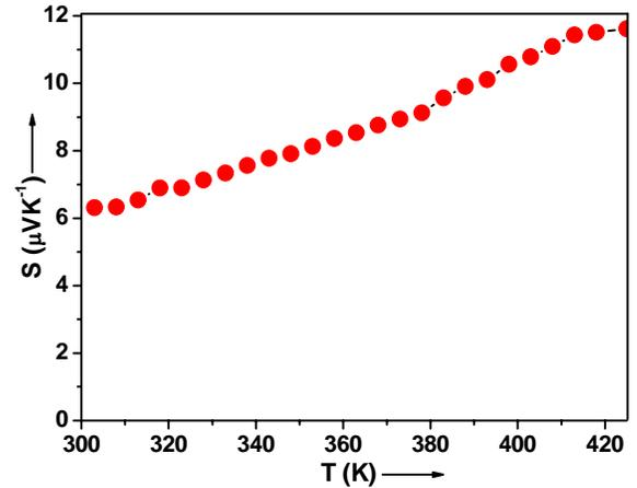
Fig. 1 Variation of S with temperature of  $\text{Cu}_7\text{Se}_4$  film
