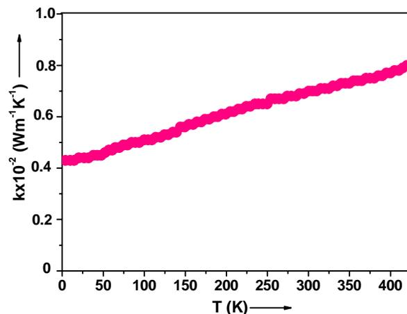
Fig. 12 Variation of  $k$  with temperature of InSe film
