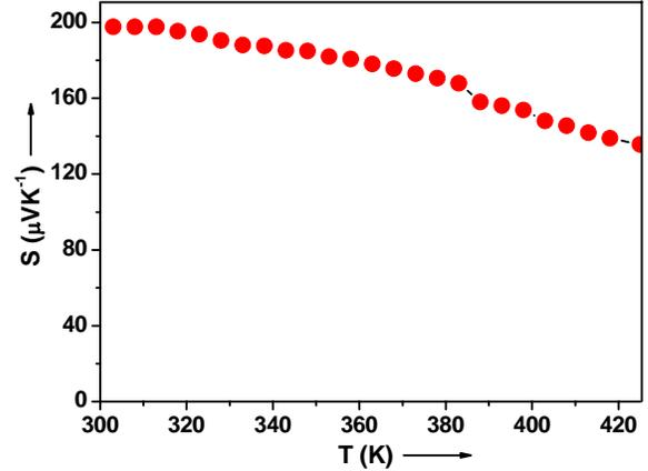
Fig. 4 Variation of  $S$  with temperature of InSe film
