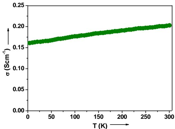
Fig. 9 Variation of  $\sigma$  with temperature of InSe film
