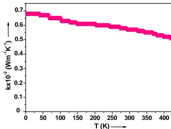
Fig. 11 Variation of  $k$  with temperature of  $\text{Cu}_7\text{Se}_4$  film
