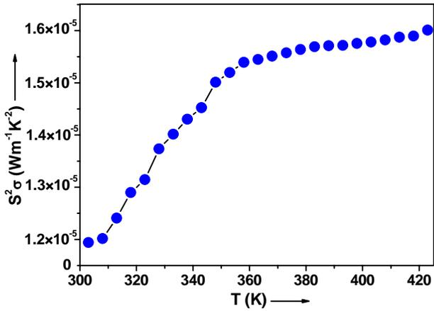
Fig. 3 Variation of  $S^2\sigma$  with temperature of  $\text{Cu}_7\text{Se}_4$  film
