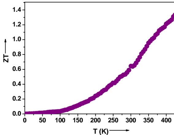
Fig. 13 Variation of ZT with temperature of  $\text{Cu}_7\text{Se}_4$  film
