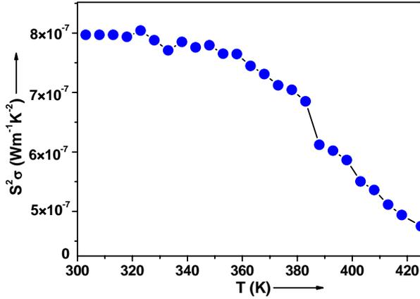
Fig. 6 Variation of  $S^2\sigma$  with temperature of InSe film
