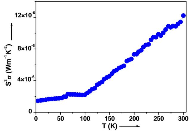
Fig. 8 Variation of  $S^2\sigma$  with temperature of  $\text{Cu}_7\text{Se}_4$  film
