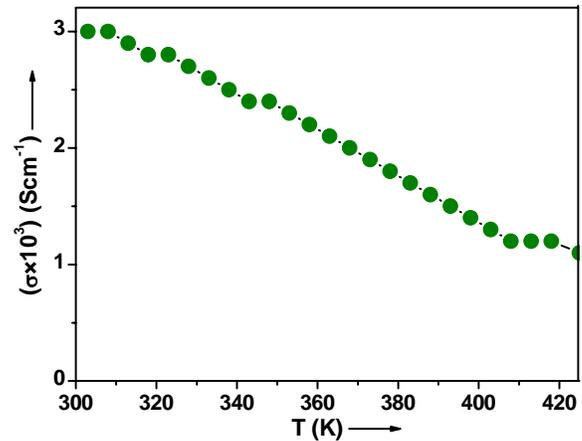
Fig. 2 Variation of  $\sigma$  with temperature of  $\text{Cu}_7\text{Se}_4$  film
