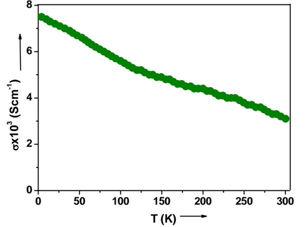
Fig. 7 Variation of  $\sigma$  with temperature of  $\text{Cu}_7\text{Se}_4$  film
