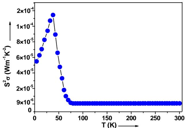
Fig. 10 Variation of  $S^2\sigma$  with temperature of InSe film
