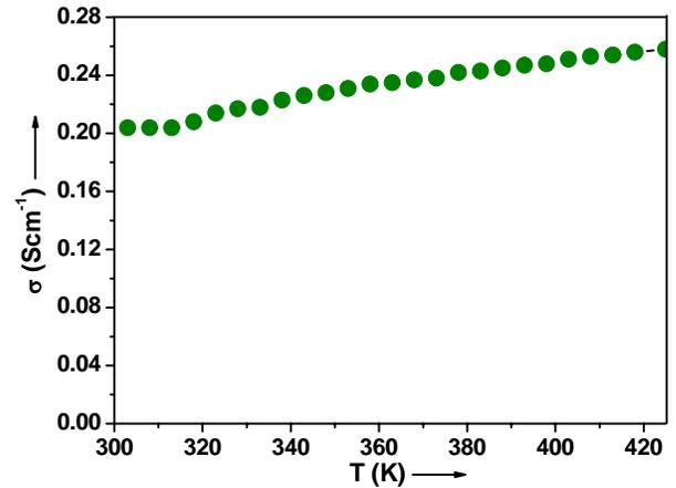
Fig. 5 Variation of  $\sigma$  with temperature of InSe film
