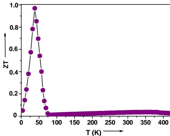
Fig. 14 Variation of ZT with temperature of InSe film
